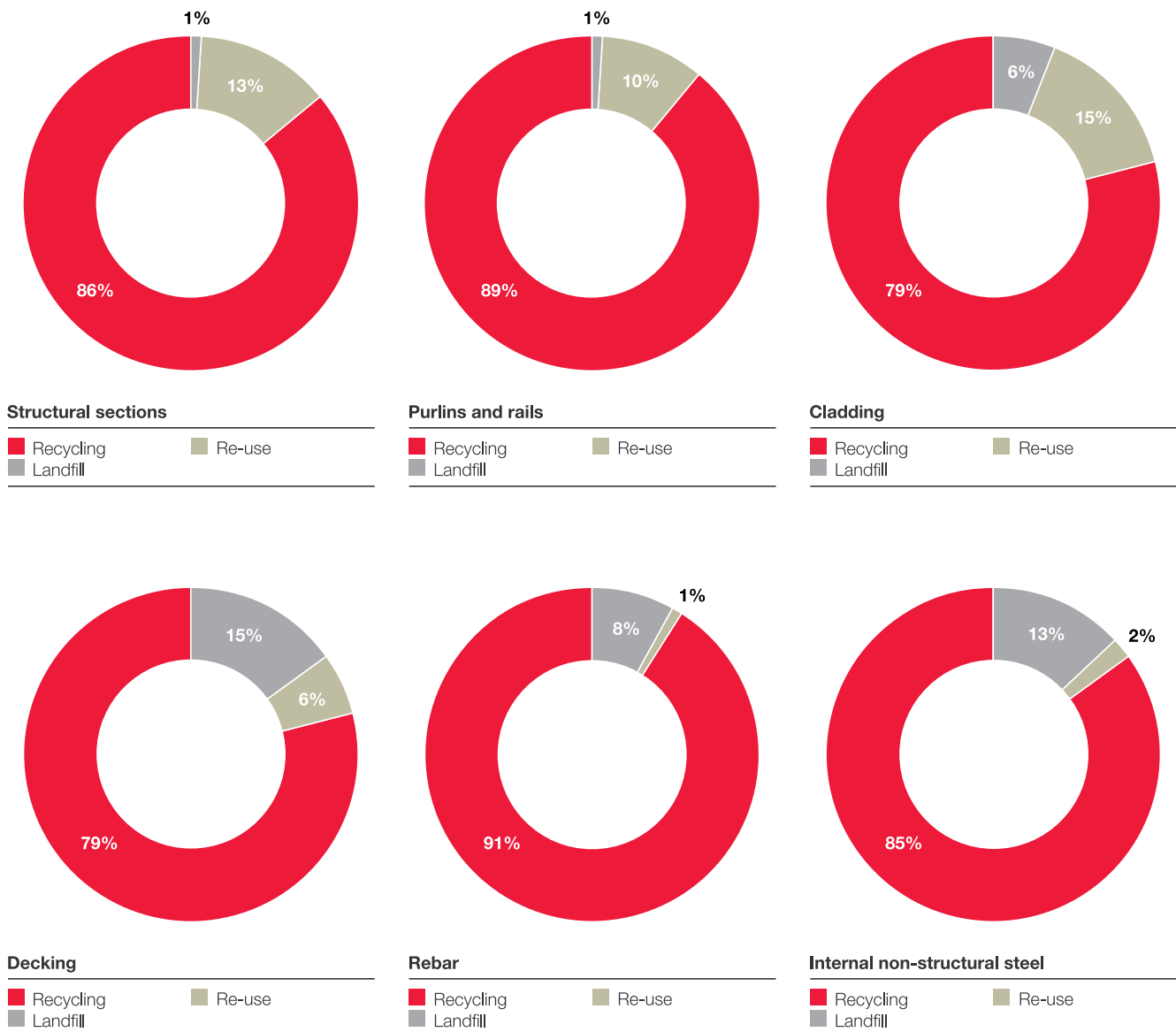
Fig. 1. Re-use and recycling of constructional steel
